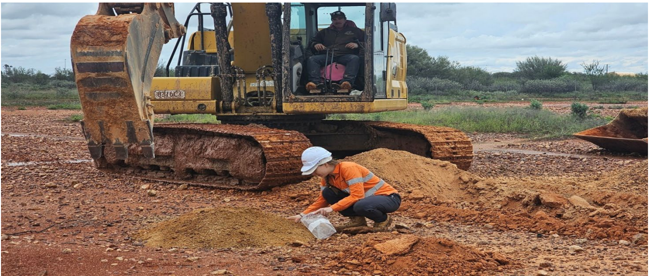
Douglas Partners - Soil testing STP site
